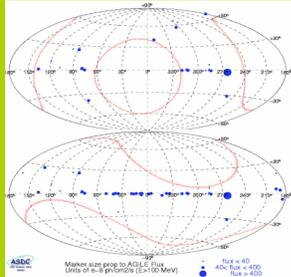
Figure 2: Sky map in HAMMER-AITOFF projection in Galactic coordinates showing the portion of sky accessible by AGILE in Spinning Mode at two different dates: 2013/01/01 and 2013/04/01. Red lines show exclusion regions around the Sun and Anti-Sun. The First Agile Catalogue Sources [8] are also shown.
