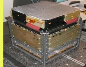
Figure 1: the AGILE payload. The gamma-ray imager GRID and, on top of it, the hard X-ray Super-AGILE detector.
